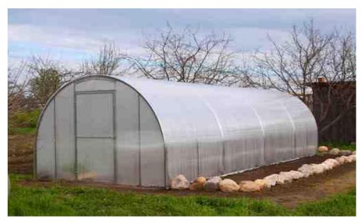
'Polyhouse is a type of greenhouse which is covered using a thin sheet of polyethylene (cladding material).'
